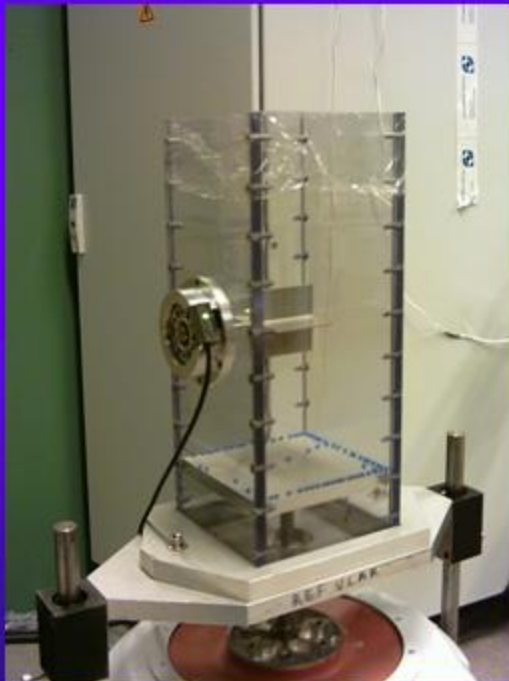
Precision rotational sensor: 4.8 \cdot 10^{-6} rad
